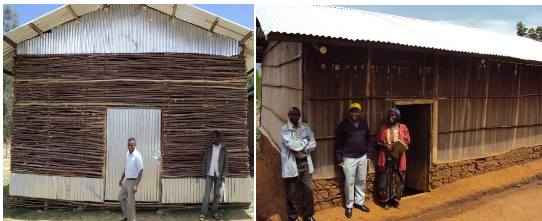
Plate 4. Diffused light stores constructed in (a) Ethiopia and (b) in Uganda. The one in Uganda is fitted with aphid proof nets.
