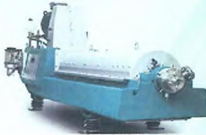
Decanter: A machine to separate the potato protein from the starch and pulp for additional value such for animal feed in the fattening program
