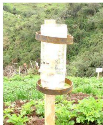
Photograph 3.3.3. Domestic rain collector made with a plastic bottle.
