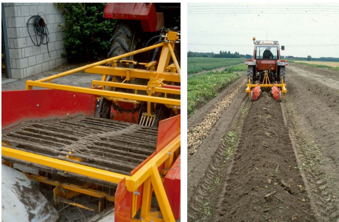
Figure 8.13. Lifter which is lifting two ridges and which is putting the tubers in one row (left) and the machine which is covering the lifted tubers with soil.
