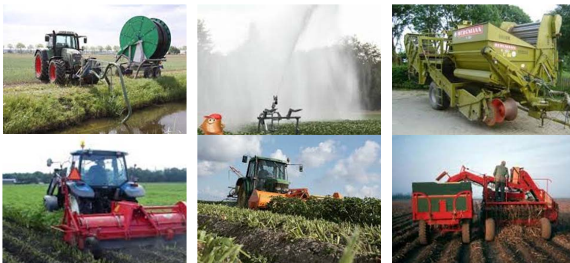
Figure 2.3. Some examples of mechanisation options for the potato cultivation in India. Above left and middle: tractor supported spray gun irrigation; above right: a one row harvest bunker; below left: haulm shredder; middle: haulm topper; right: harvest directly loading on truck.
