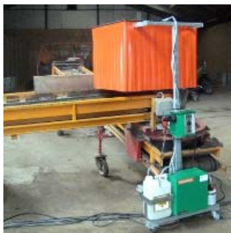
Figure 8.12. Spinning disk atomizer (Mafex) attached on a rolling table.
